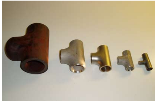
Figure 5.7.1 Connection pieces made by hydroforming are shown on the right. On the left, an operational solution for the use of hydroformed parts as components in a power transmitting structure. /Oy OSTP Ab/.
