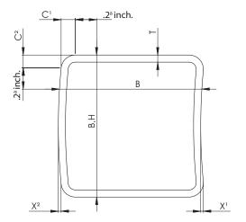
$^{\rm a}$  This dimension is maximum when measuring B or H and minimum when measuring T
