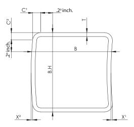
$^{\rm a}$  This dimension is maximum when measuring B or H and minimum when measuring T
